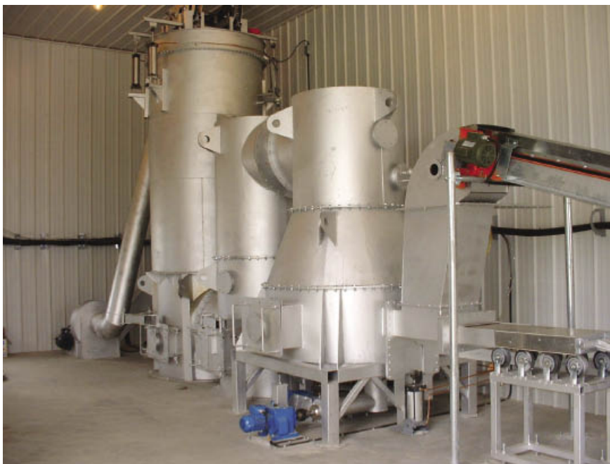
A three-million-BTU biomass burner made by Triple Green Energy in St. Adolphe. The heating units can
